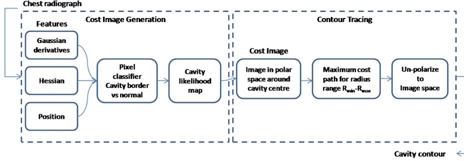
Fig. 1. Proposed cavity contour segmentation approach
